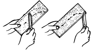
The entire bevel face should come in contact with the abrasive surface:
